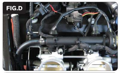
Attach the connectors from the PCFC harness to the stock wiring harness and injectors as shown in Figure D.
