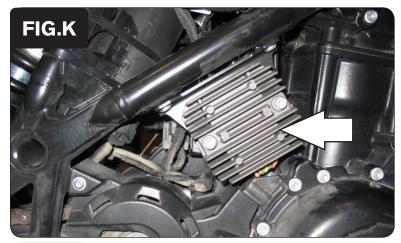
16 Remove the regulator/rectifier to access the O2 sensor connection as shown in Figure K.
