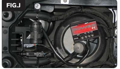
Using the supplied velcro, secure the PCFC as shown in Figure J.Make sure to clean both surfaces with the alcohol swab before attaching.
