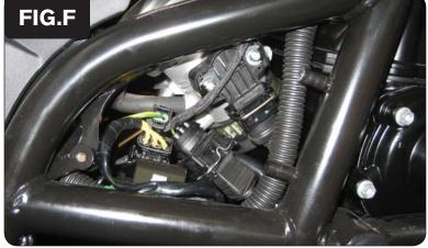
1 Attach the connectors from the PCFC harness to the stock wiring harness and Throttle Position Sensor as shown in Figure F.
