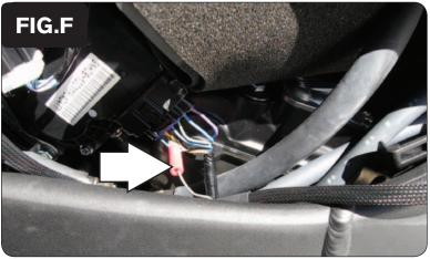
12 Using the supplied posi-tap, attach the grey wire from the PCFC to the blue/black wire of the stock Throttle Position Sensor (TPS) harness.
