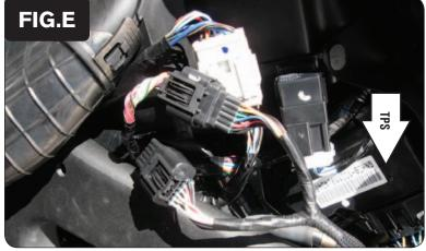
11 Attach the PCFC connectors to the stock connectors as shown in Figure E.
