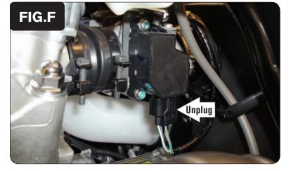
At the left side of the throttle body, unplug the stock wiring harness from the ATV's Throttle Position Sensor (Fig. F).
