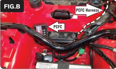
2 Using the supplied Velcro, secure the PCFC module towards the front of the battery compartment.
