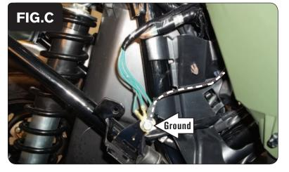
Inside of the right-rear fender well, secure the PCFC ring lug to the common ground bolt on the frame (Fig. C).
