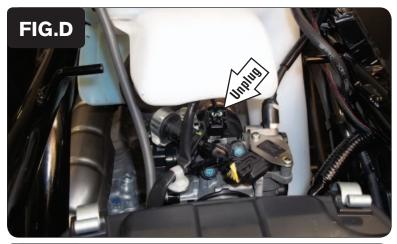
At the top of the throttle body, unplug the stock wiring harness from the ATV's Fuel Injector (Fig. D).
