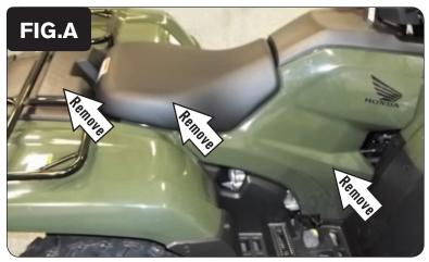
1 Remove the seat, the battery cover rear of the seat, and the body panels surrounding the ATV's fuel tank (Fig. A).
