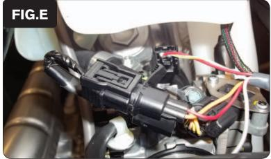
Plug the PCFC wiring harness in-line of the Fuel Injector and the stock wiring harness (Fig. E).
