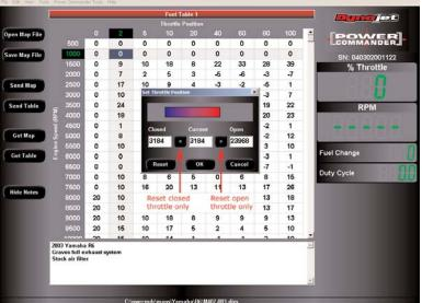
To reset both the closed and open throttle positions, first make sure that the bike is communicating to the computer, then click on "Reset". Twist the throttle wide open and release. Now click OK.
