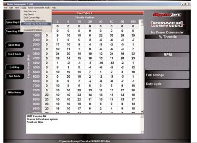
If you want to change the resolution of a map from 500rpm to 250rpm go into "Tools" and select "Maximize Map Resolution".
