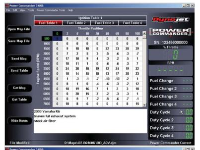
"Advanced Mode" displays individual cylinder mapping and shows "Fuel Change" and "Duty Cycle" for each cylinder.
