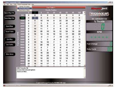
To reset the throttle position click on "Power Commander Tools" and then select "Set Throttle Position
