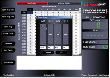
In the "Cylinder Trims" window, click and drag the sliders to adjust each individual cylinder. This screen shows that Cylinder #1 is made 5% richer than the base map.
