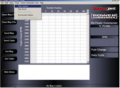
"Map Compare" can be used to view the differences between two map files. To access this feature, click on "Tools" on the menu bar and select "Map Compare."
