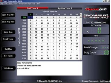
The monitor function in standard mode displays the throttle position in "real time." At idle (when the bike is at full operating temperature) the "% Throttle" value should read "0." At wide open throttle, it should read "100." Engine RPM is also displayed along with the current fuel change based on the "% Throttle" and "RPM" combination. "Duty Cycle" displays the percentage of time the injector is open during one cam revolution.
