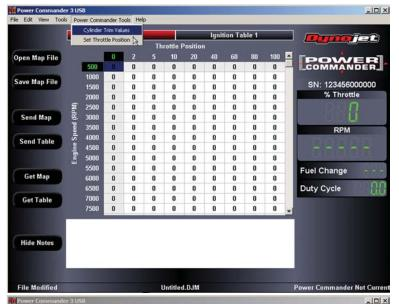
To offset the fuel curve to different cylinders, use the Cylinder Trim Function by clicking on "Power Commander Tools" on the menu bar and selecting "Cylinder Trim Values."
