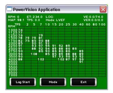
AutoTune Datalogger monitors various operating conditions to ensure you're ready to start auto tuning and whether or not you're in a state to allow learning. A large message will overlay the screen to indicate the condition that's currently preventing learning. Refer to <u>AutoTune Datalogger Operating Conditions</u> for a list of conditions.
