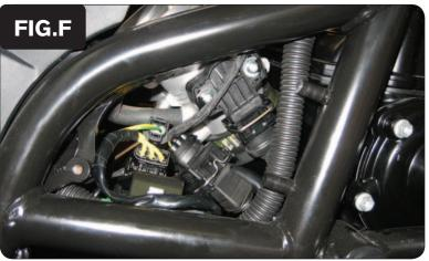
Plug the PCV wiring harness in-line of the stock wiring harness and both of the fuel injectors (Fig. D).
