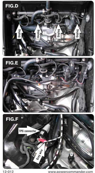
8 Unplug the stock wiring harness from each fuel injector (Fig. D).
