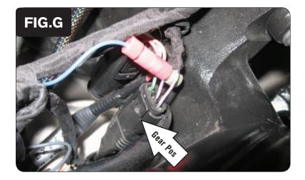
12 Using the other supplied Posi-tap, connect the BLUE/WHITE wire of the PCV to the stock PURPLE/BLACK wire of the gear position sensor connector (Fig. G).
