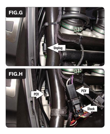
10 Unplug the stock wiring harness from the Throttle Position Sensor (Fig. G). This sensor is located on the left side of the throttle bodies.
