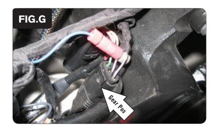
12 Using the other supplied Posi-Tap, connect the BLUE/WHITE wire of the PCV to the stock PURPLE/BLACK wire of the gear position sensor connector (Fig. G).
