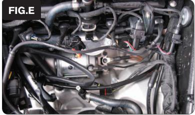
9 Plug the PCV harness in-line of the stock wiring harness and each fuel injector (Fig. E).
