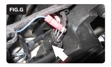
12 Using the supplied Posi-Tap connect the BLUE wire of the PCV to the PUR/BLK wire of the gear position sensor connector (Fig. G).
