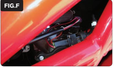
Plug the pair of PCV leads with ORANGE colored wires in-line of the front fuel injector and the stock wiring harness (Fig. F).
