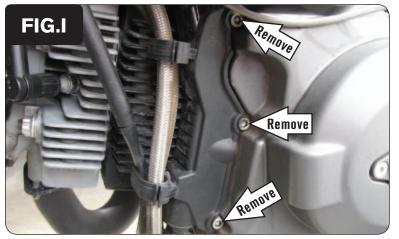
12 Remove the BLACK plastic engine cover on the left side of the bike by removing the 3 bolts (Fig. I).
