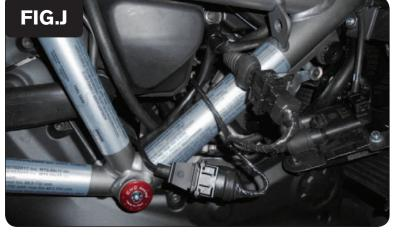
17 Plug the pair of matching PCV connectors in-line of the stock Crank Position Sensor connectors (Fig. J).
