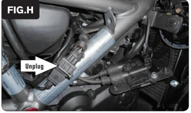
16 Unplug the Crank Position Sensor connectors on the right hand side of the bike (Fig. H).
