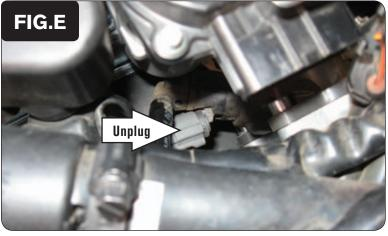
Unplug the stock wiring harness from the rear fuel injector (Fig. E).
