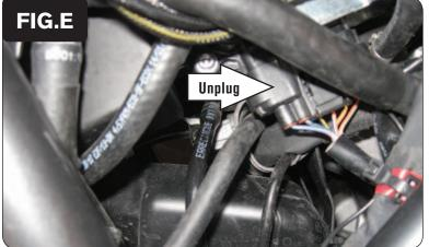
10 Unplug the Throttle Position Sensor connector from the main wiring harness (Fig. E).
