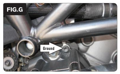
12 Attach the ground wire of the PCV with the small ring lug to an engine case bolt on the left side (Fig. G).
