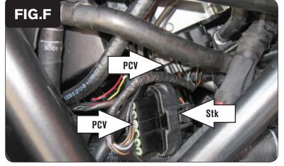
Plug the PCV in-line of the TPS and the stock wiring harness (Fig. F).
