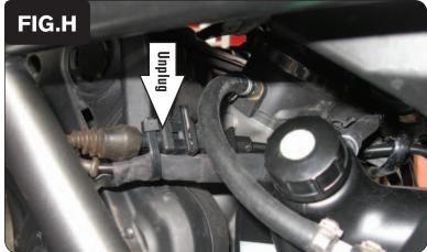
13 Locate and unplug the stock Crank Position Sensor connectors (Fig. H).
