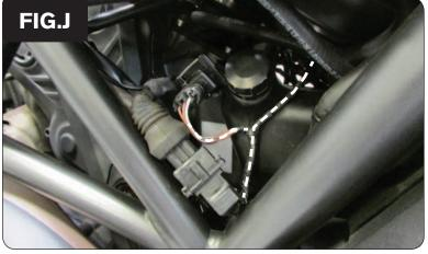
14 Plug the pair of matching PCV connectors in-line of the stock Crank Position Sensor connectors (Fig. J).
