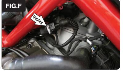
Locate and unplug the stock Crank Position Sensor connectors on the left side of the engine (Fig. F).
