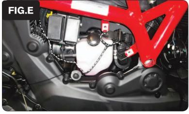
8 Plug the PCV in-line of the stock CPS connectors (Fig. E).
