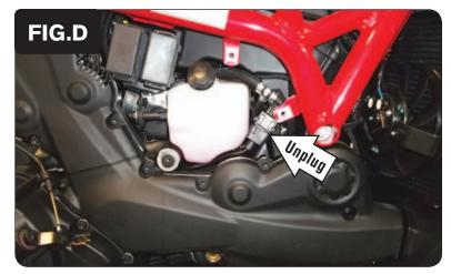
7 Unplug the stock Crank Position Sensor connectors (Fig. D).
