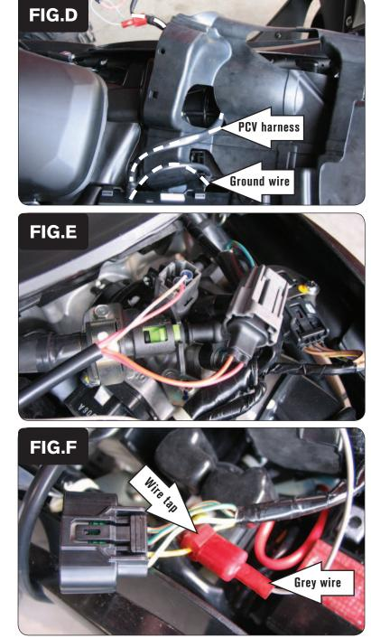
5 Route the PCV harness thru the rubber cover as shown in Figure D.
