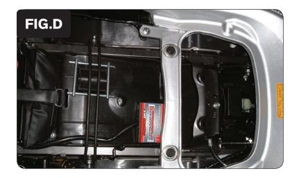
Install the PCV in the tail section using the supplied velcro to secure the unit in place (Fig. D).
