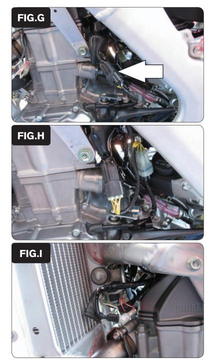
8 Unplug the crank position sensor connector (Fig. G). This is a BLACK 6 pin connector on the left side of the motorcycle.
