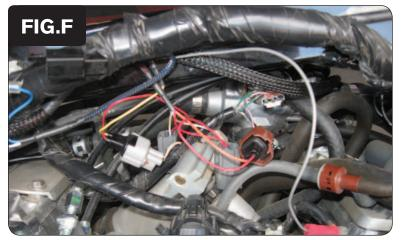
10 Route the remainder of the PCV wiring harness towards the right hand side of the bike, through the frame, under the fuel tank, and towards the throttle bodies while following the stock wiring harness on the right hand side of the frame as closely as possible.
