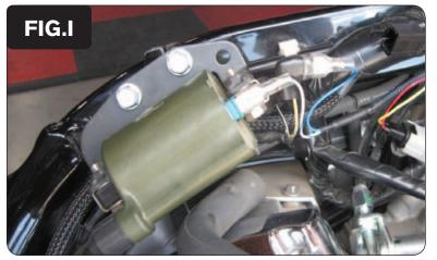
Plug the pair of BLUE colored wires of the PCV in-line of the Rear Ignition Coil's GREEN spade and the stock YELLOW/BLUE wire (Fig. I).
