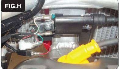
10 Plug the PCV wiring harness in-line of the ignition coil and the stock coil wires (Fig. H).
