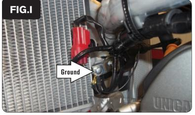
11 Secure the ground wire of the PCV wiring harness with the 6mm ring lug to the stock ground location (Fig. I).
