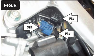
7 Plug the PCV harness in-line of the stock TPS and wiring harness (Fig. E)
