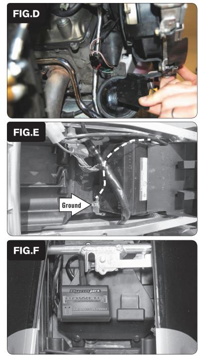
7 Plug the pair of 2-pin PCV connectors in-line of the stock Crank Position Sensor connectors (Fig. D).
