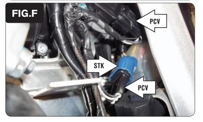
Plug the PCV wiring harness in-line of the TPS and the stock wiring harness (Fig. F).
