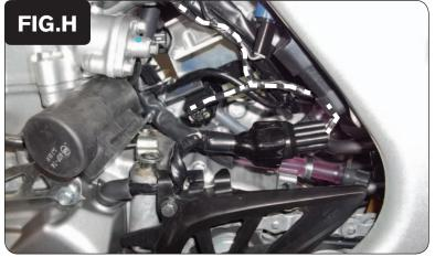
10 Plug the PCV wiring harness in-line of the stock Crank Position Sensor connectors (Fig. H).
