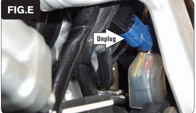
7 Unplug the stock wiring harness from the Throttle Position Sensor on the left side of the throttle body (Fig. E).
