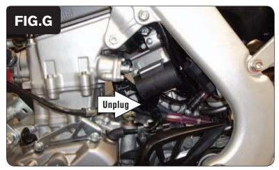
9 Locate and unplug the stock connectors from the bike's Crank Position Sensor (Fig. G).
