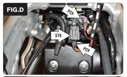
Plug the pair of PCV leads with ORANGE colored wires in-line of the Fuel Injector and the stock wiring harness (Fig. D).
