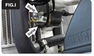
11 Unplug both of the stock coil wires (Fig. I).
