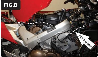
2 Loosen the front of the fuel tank. Lift and prop the fuel tank in an upright position.
