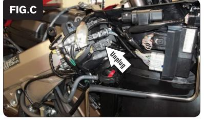
Locate and unplug the stock fuel injector sub-harness connectors (Fig. C).
