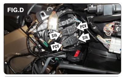
5 Plug the mating pair of 12-pin PCV connectors in-line of the stock fuel injector sub-harness connectors (Fig. D).
