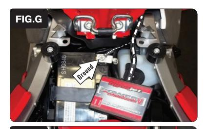
8 Secure the PCV ground wire with the small ring lug to the negative (-) terminal of the bike's battery (Fig. G).
