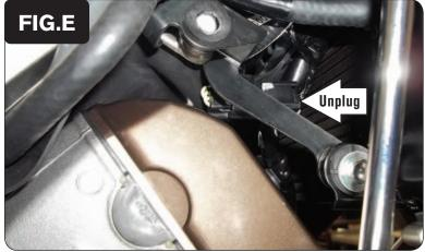
6 Locate and unplug the stock Crank Position Sensor connectors (Fig. E).
