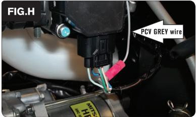
Use the supplied Posi-tap, to attach the PCV single unterminated GREY wire to the stock BLACK/BLUE wire of the TPS connector.
