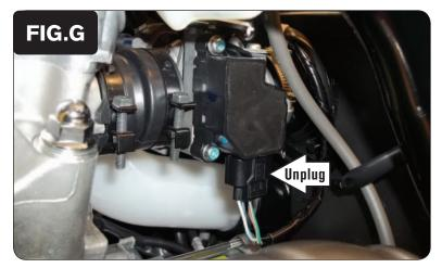
12 At the left side of the throttle body, unplug the stock wiring harness from the ATV's Throttle Position Sensor (Fig. G).
