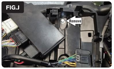
15 Pull the ECM rearward and unlatch it from its mounting bracket. Remove the bolt found beneath the ECM (Fig. J).
