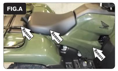
Remove the seat, the battery cover rear of the seat, and the body panels surrounding the ATV's fuel tank (Fig. A).
