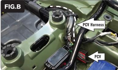
2 Using the supplied Velcro, secure the PCV module to the right side of the compartment directly in front of the battery.
