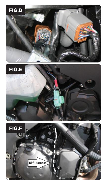
5 Connect the PCV in-line of the stock wiring harness and throttle body harness (Fig. D).
