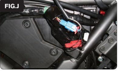
14 Plug the PCV in-line of the stock wiring harness and CPS (Fig. J).
