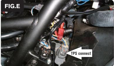
This picture was taken with the coolant bottle moved out of the way
