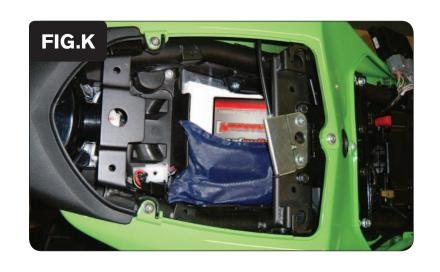
Using the supplied velcro, secure the PCV unit in the tail section (Fig. K).
