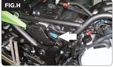
13 Unplug the Crank Position Sensor from the stock wiring harness (Fig. H).
