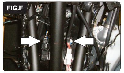
The coil sticks are located on top of the engine. In Figure F the #1 (left) coil stick is located under the Baro pressure sensor.
