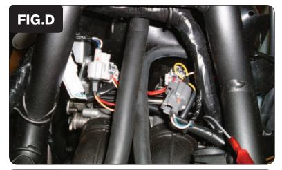
Plug the PCV harness in-line of the stock wiring harness and injectors (Fig. D).
