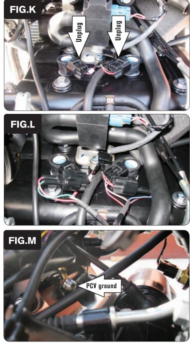
11 Unplug the stock wiring harness from the coil sticks (Fig. K).
