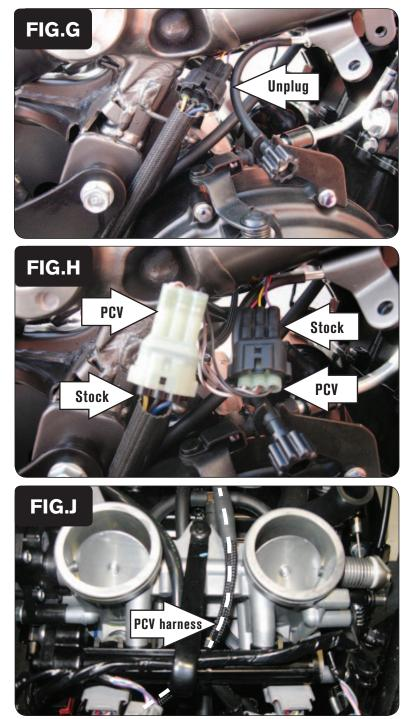
8 Locate and unplug the bike's Crank Position Sensor connectors on the righthand side of the bike (Fig. G).
