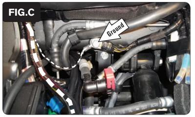
5 Secure the PCV ground wire with the small ring lug to the common ground location at the center of the frame just rear of the engine (Fig. C).
