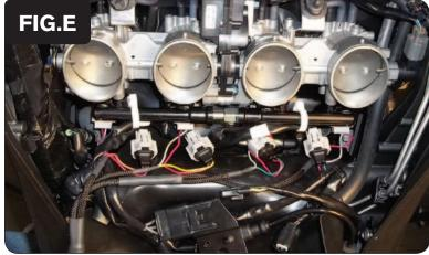
Plug the PCV wiring harness in-line of each injector and the stock wiring harness (Fig. E).
