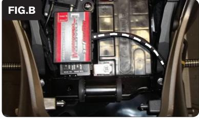
3 Using the supplied Velcro, secure the PCV module under the seat and next to the battery (Fig. B).
