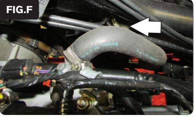
7 Locate the Ignition coil (Fig. F).
