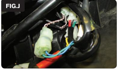
10 Plug the PCV in-line of the stock CPS and wiring harness (Fig. J).
