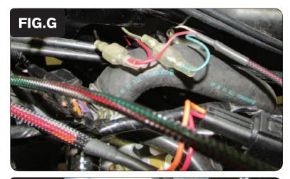
8 Plug the PCV harness in-line of the stock coil and wiring harness (Fig. G).
