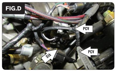
5 Plug the PCV in-line of the TPS and wiring harness (Fig. D).
