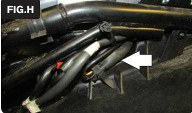
9 Locate the Crank Position Sensor connector (Fig. H).
