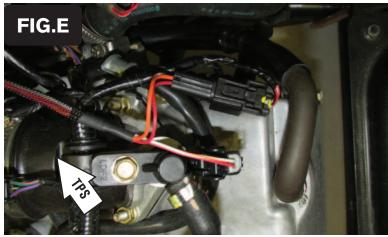
6 Plug the PCV harness in-line of the stock injector and wiring harness (Fig. E)
