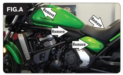
1 Remove the seat, the left side panel, the key switch cover. Remove the left and right side knee panels (Fig. A).
