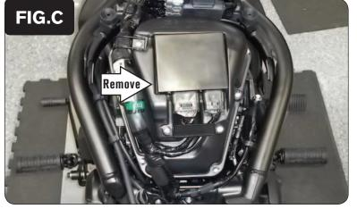
Remove the ECU and loosen the stock wiring from the airbox. Remove the airbox (Fig. C).
