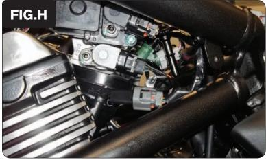
Plug the PCV wiring harness in-line of the lower primary Throttle Position Sensor and the stock wiring harness (Fig. H).
