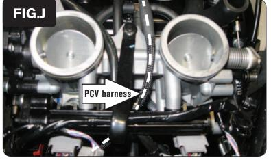
10 Route the remainder of the PCV wiring harness with the coil connectors under the fuel rail, in between the throttle bodies, and up towards the coil sticks (Fig. J).
