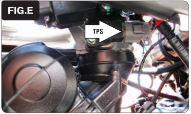
Locate and unplug the stock wiring harness from the Throttle Position Sensor on the left hand side of the bike's throttle bodies (Fig. E).
