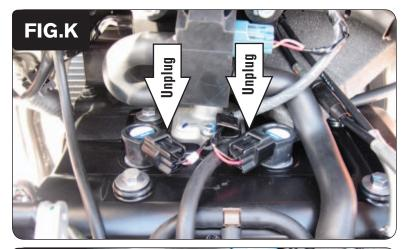
11 Unplug the stock wiring harness from the coil sticks (Fig. K).
