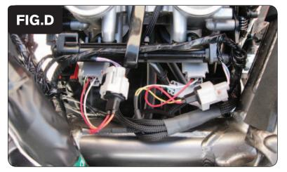
5 Plug the PCV connectors in-line of the stock wiring harness and fuel injector for both cylinders (Fig. D).
