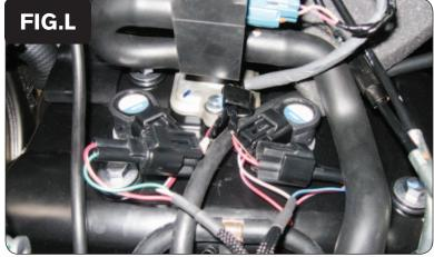
12 Plug the PCV wiring harness in-line of the stock wiring harness and the coil sticks (Fig. L).
