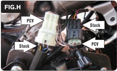
9 Plug the PCV connectors in-line of the stock Crank Position Sensor connectors (Fig. H).
