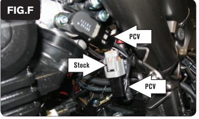
Plug the PCV wiring harness in-line of the stock wiring harness and the TPS (Fig. F).
