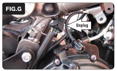
8 Locate and unplug the bike's Crank Position Sensor connectors on the right-hand side of the bike (Fig. G).
