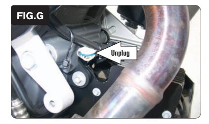
12 Locate the stock Crank Position Sensor connectors under the chin fairing at the front of the motorcycle (Fig. G).
