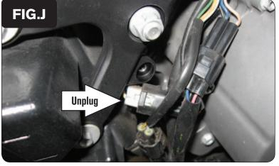
This is a 2-pin connector pair. The MALE connector is WHITE. The FEMALE connector is BLACK.
