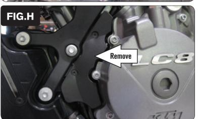
13 Remove the small plastic cover on the left side of the engine (Fig. H).
