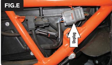
8 Locate the stock connector from the throttle bodies on the right side of the motorcycle. Unplug this connector (Fig. E).
