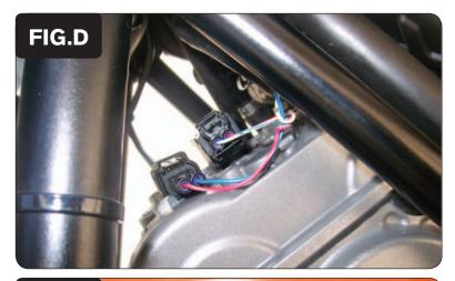
Plug the pair of PCV connectors with BLUE colored wires in-line of the Rear Ignition Coil and the stock wiring harness (Fig. D).
