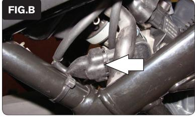
3 Unplug the stock Throttle Position Sensor connector (Fig. B).
