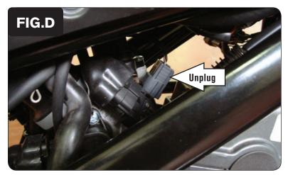
5 Unplug the wiring harness from the fuel injector (Fig. D).
