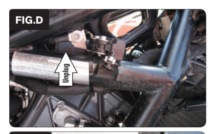
8 Locate the sub-harness connectors from the throttle bodies on the right side of the motorcycle. Unplug this connection (Fig. D).
