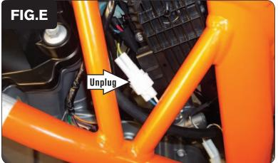
Once the Throttle Body Servo is unplugged, locate and unplug the stock Crank Position Sensor connectors just in front of the Throttle Body Servo (Fig. E).
