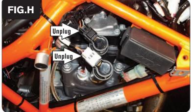
14 On the right side of the engine, locate and unplug the stock BLACK 2-pin connector from the inner coil stick and the stock WHITE 2-pin connector from the outer coil stick (Fig. H).
