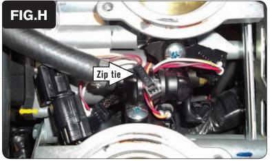
9 Plug the PCV harness in-line of the stock wiring harness and both fuel injectors (Fig. H).
