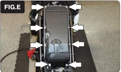
6 Remove the airbox cover by removing the 8 bolts for the lid (Fig. E).
