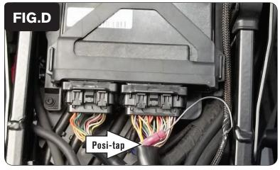
Using the supplied Posi-tap secure the GREY wire of the PCV to the stock ORANGE/YELLOW wire of the larger ECU connector (Fig. D).
