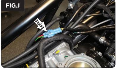
11 Unplug the stock wiring harness from the Crank Position Sensor (Fig. J).
