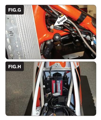
11 Secure the PCV ground wire with the small ring lug to the common ground location on the frame (Fig. G).
