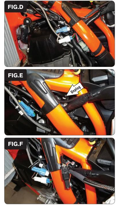
8 Plug the PCV wiring harness in-line of the stock Crank Position Sensor connectors (Fig. D).
