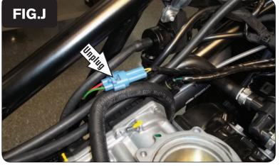
11 Unplug the stock wiring harness from the Crank Position Sensor (Fig. J).
