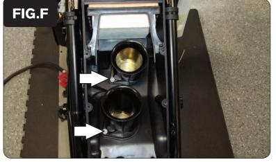
Remove the airbox by removing the 4 bolts for the velocity stacks (Fig. F).
