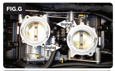
8 Unplug the stock wiring harness from both of the fuel injectors (Fig. G).
