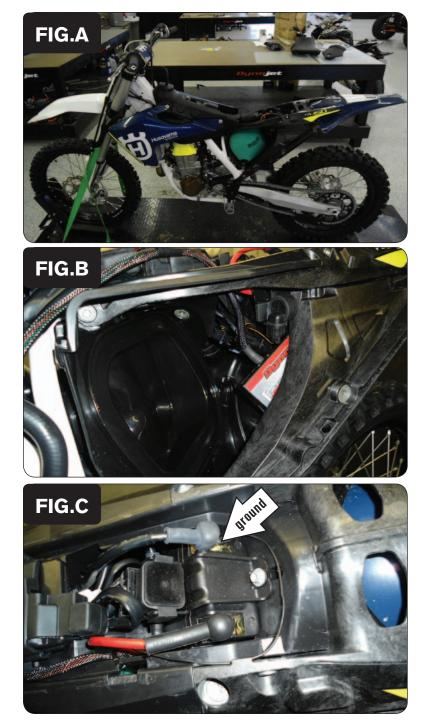
1 Remove the side panels, seat, shrouds, and fuel tank.
