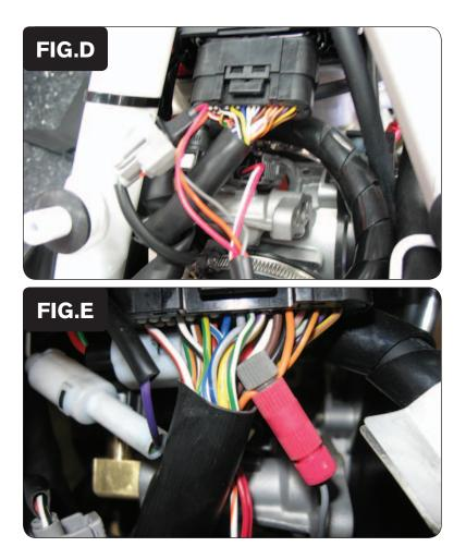
7 Plug the PCV wiring harness in-line of the stock wiring harness and fuel injector (Fig. D).
