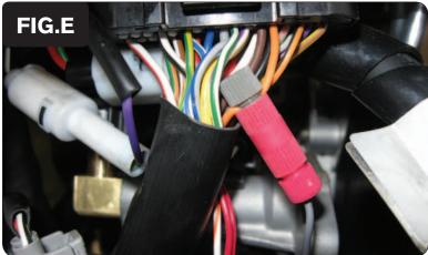
Using the supplied Posi-tap, attach the GREY wire of the PCV to the stock ORANGE wire of the main wiring harness plugged in at the ECU (Fig. E).
