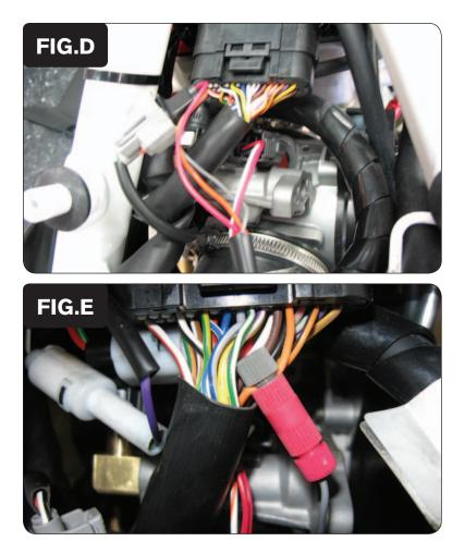
7 Plug the PCV harness in-line of the fuel injector and the stock wiring harness (Fig. D).
