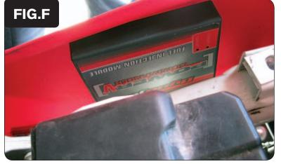
11 Using the supplied Velcro, attach the PCV module to the inside of the left radiator shroud (Fig. F).
