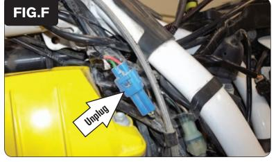
10 Unplug the bike's Crank Position Sensor connectors (Fig. F).
