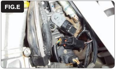
9 Plug the pair of 3-pin PCV connectors in-line of the TPS and the stock wiring harness (Fig. E).
