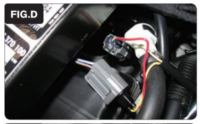
6 Plug the pair of PCV leads with YELLOW colored wires in-line of the stock wiring harness and the rear fuel injector (Fig. D).
