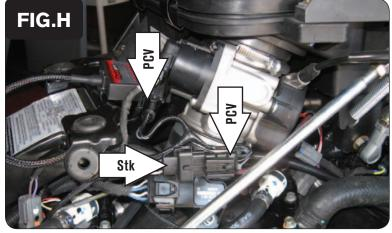
12 Plug the PCV connectors in-line of the stock wiring harness and TPS (Fig. H).
