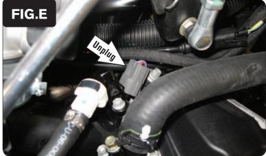
7 Unplug the stock wiring harness from the front fuel injector (Fig. E).
