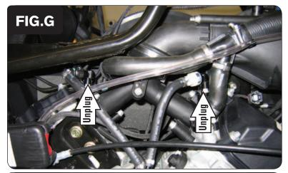
11 Locate and unplug the fuel injectors above the engine (Fig. G).
