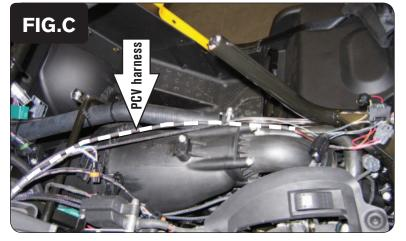
Route the PCV harness over the engine cover and along the intake plenum (Fig. C).
