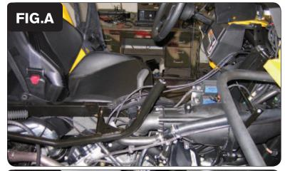
1 Remove the center console, glove compartment, ignition switch board, and both passenger side engine compartment cover panels.
