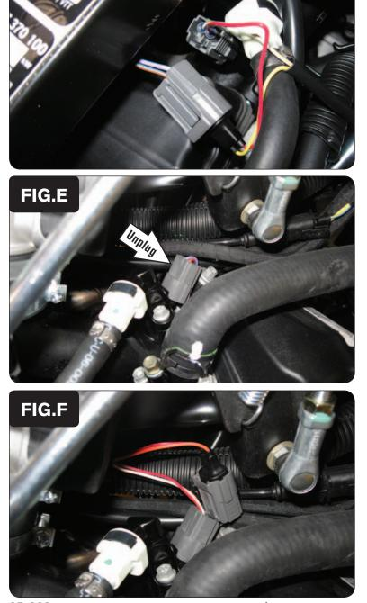
6 Plug the pair of PCV leads with YELLOW colored wires in-line of the stock wiring harness and the rear fuel injector (Fig. D).
