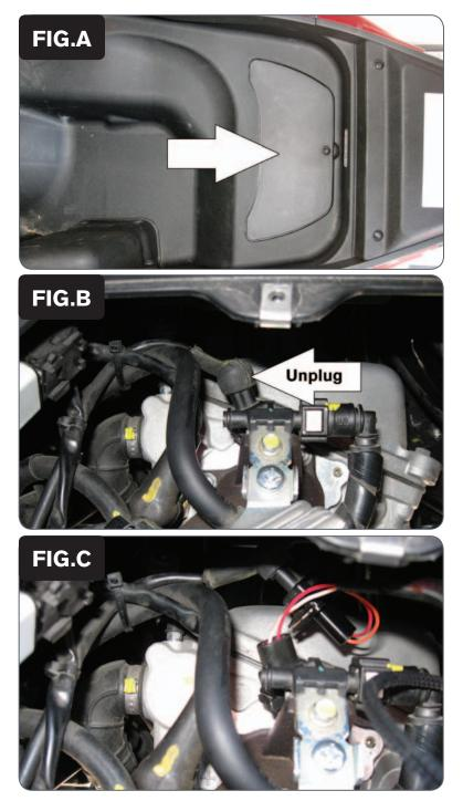
Remove the inner storage compartment cover (Fig. A).
