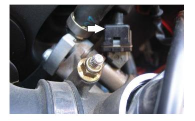
Unplug the stock wiring harness from the rear fuel injector.
