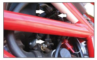
8 Unplug the stock wiring harness from the front fuel injector.
