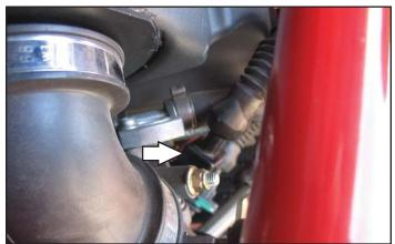
9 Plug the pair of PC6 leads with ORANGE colored wires in-line of the front fuel injector and the stock wiring harness.
